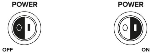
Flip the switch on the back of your speaker to the ON position to the right of the panel.
